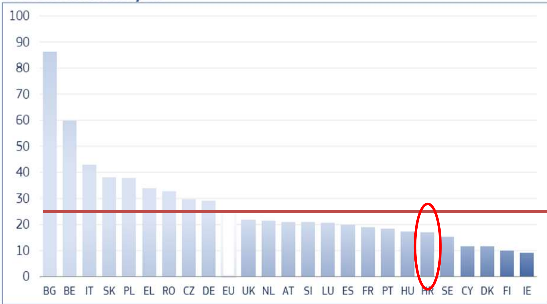
Figure 10: Motorway fatality rates per 1.000 km of motorway by country, 2014 or latest available year
